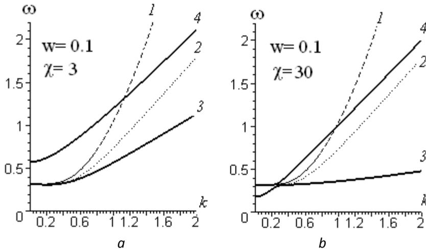
Fig. 1 Dispersion curves for frequency  $\omega-k$  for beam on elastic foundation  $w = 0,1$  in cases  $\chi = 3$  (a) and  $\chi = 30$  (b). Two branches for TB (bold curves), curves for E-B (1) and Rayleigh models (2)
