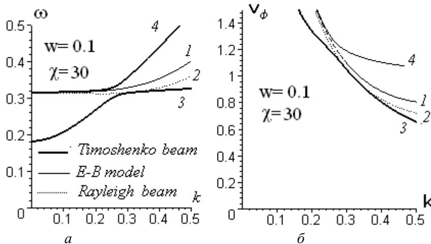
Fig. 2. Dispersion curves for frequency  $\omega-k$  (a) and phase velocity  $v_\phi-k$  (b) for beam on elastic foundation,  $w = 0,1$ ,  $\chi = 30$ , on a large scale. Two branches for TB (curves 3, 4), curves for E-B (1) and Rayleigh models (2)
